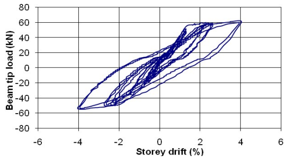
Fig. 11. Beam tip load-storey drift relationship of specimen JBC1.
